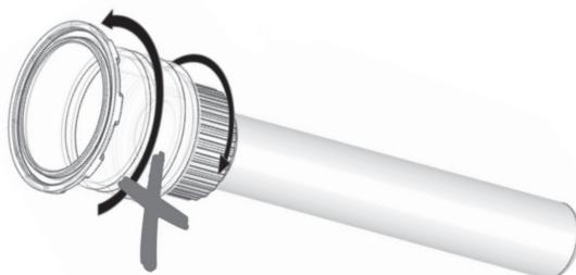
**EN: Do not disassemble!** The quartz glass connection cannot and may not be dismantled. Disassembly attempts can lead to leakage, glass breakage or personal injury. Damage to the UV-C device as a result of dismantling is not covered by the warranty.
