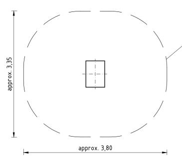
\*minimum space requirements approx. 11 m<sup>2</sup> only referring to a free-standing water wheel as illustrated. If further water play elements are added (like e.g. a water trough), space requirements will have to be adjusted.
